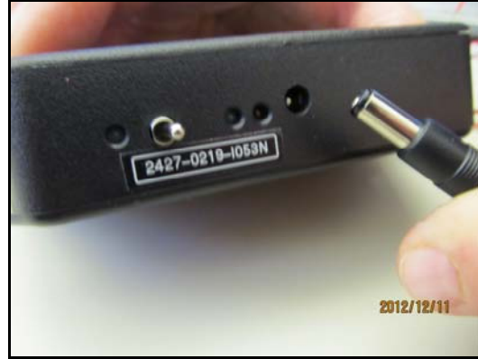
Figure 3: Installing external power barrel connector into power jack
