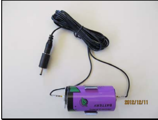
Figure 2: D-cell, battery holder and barrel connector
